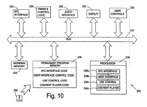
Figure 10 is a schematic diagram of data access device 220.
