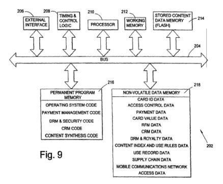
Figure 9 is a schematic diagram of the components of portable data carrier 202. Portable data carrier 202 is shown as a "smart Flash card." *Id.* at 17:6–8.
