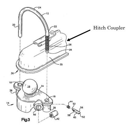
13. As the '686 patent explains, the lock blocks a would-be thief from engaging his vehicle's hitch ball with the coupler and towing the trailer away.
