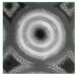
High-Angle Annular Dark-Field (HAADF) image of Micron DDR4 DRAM capacitor
