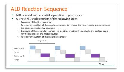
This is further illustrated by the process schematic, below, which shows a basic gas flow sequence to the chamber for Chemical Vapor Deposition and for ALD.<sup>18</sup>
