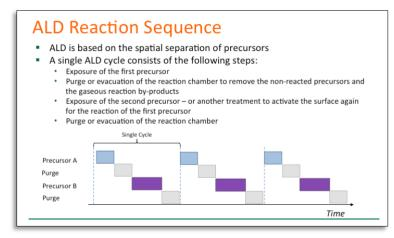
This is further illustrated by the process schematic, shown below, which shows a basic gas-flow
