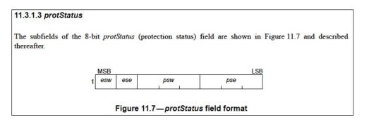
11.3.1.3.1 esw: A (edge state, west) bit that indicates whether an edge is present on the west span of a station. A value of 0 indicates that there is no edge, whereas a value of 1 indicates that an edge is present.
