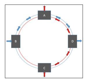
54. The dual-ring topology provides robustness by including the capability of automatic reconfiguration after a link failure. If a node on the ring or a link between two nodes is disrupted or fails, traffic can be looped back around the ring in the opposite direction to the destination node and avoid the disruption/failure.
