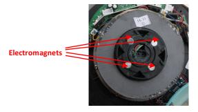
g. The Accused Product has a controller located within the base, which controller is connected to the position sensor system and the electromagnets, receives signals from the position sensor system, and controls the electromagnets in response to such signals.
