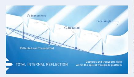
inward and only some is refracted outward. At about 42 degrees to the perpendicular, all the light is effectively trapped — hence "Total Internal Reflection." It doesn't matter that the acrylic is transparent. The light can't escape and will bounce down the waveguide like a billiard ball bouncing off cushions to travel along an endless billiard table.
