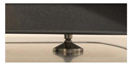
20. In one sample measuring position, the opposed substantially parallel surfaces are spaced apart (approximately 0.5 mm) to pull the sample into a column where it is contained by surface tension.
