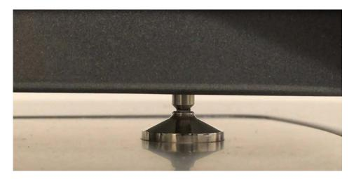
34. In one sample measuring position, the opposed substantially parallel surfaces are spaced apart (approximately 0.5 mm) to pull the sample into a column where it is contained in tension by surface tension.
