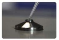
33. In the sample compression position, the upper anvil is lowered to a position selected so that the anvil surfaces are opposed and substantially parallel and proximally spaced (approximately 0.15 mm apart) so that the liquid wets and spreads upon both surfaces.
