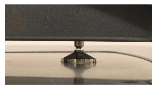
21. A measurement of the sample is then taken by directing a light from a xenon flash lamp through an optical fiber to the lower anvil and detecting the light passing through the sample through an optical fiber at the upper anvil that leads to a detector.
