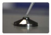
19. In the sample compression position, the upper anvil is lowered to a position selected so that the anvil surfaces are opposed and substantially parallel and proximally spaced (approximately 0.15 mm apart) so that the liquid wets and spreads upon both surfaces.
