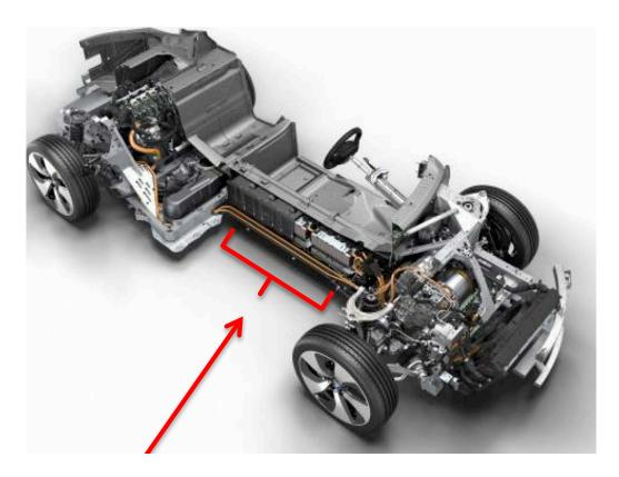
117. The BMW i8 vehicle chassis includes "a battery ... located in the energy storage compartment," as shown below:
