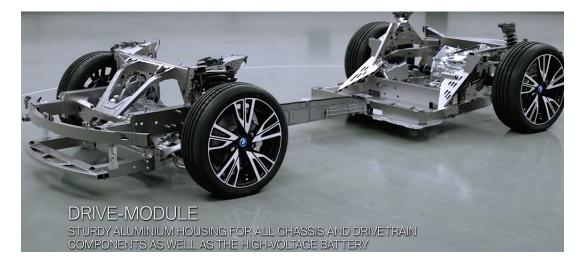
107. The BMW i8 vehicle chassis includes "a central backbone structure enclosing an energy storage compartment therein," as shown below:
