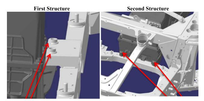
111. The BMW i8 vehicle chassis includes "a middle of the central backbone structure has a smaller lateral width than do either of the first and second structures," as shown below:
