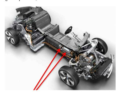
118. The "central structure" of the BMW i8 vehicle chassis "includes a closed-wall section," as shown below:
