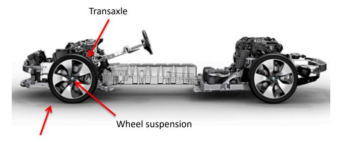
110. The BMW i8 vehicle chassis includes "the central backbone structure being rigidly attached to the first and second structures such that ride, handling and impact crash loads are primarily transmitted between the first and second structures by the central backbone structure," as shown below:
