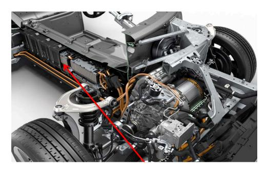
119. The "central structure" of the BMW i8 vehicle chassis "further compris[es] a removable service plate," as shown below:
