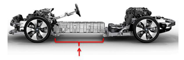
116. The BMW i8 vehicle chassis includes "an energy storage compartment located inside of the central chassis structure," as shown below:
