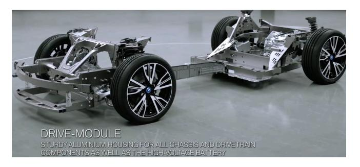
115. The BMW i8 vehicle chassis includes "an elongated and single central chassis structure longitudinally spanning between and being the sole structural connection between the front and rear wheel axes," as shown below:
