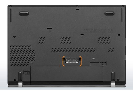
the docking-station connector containing high-speed digital signals for communicating data, address, and control to an expansion bus in the docking station (shown in aqua below), the expansion bus for receiving expansion cards to expand functions performed by the portable PC when the portable PC is connected to the docking station through the docking-station connector;
