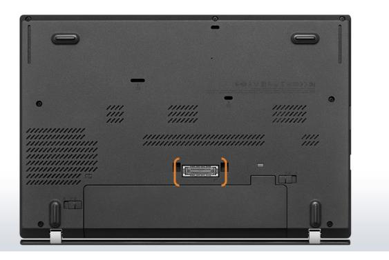
the docking-station connector means containing high-speed digital signals for communicating data, address, and control to a bus in the docking station (shown in aqua below), the bus for expanding functions performed by the portable PC when the portable PC is connected to the docking station through the docking-station connector means;
