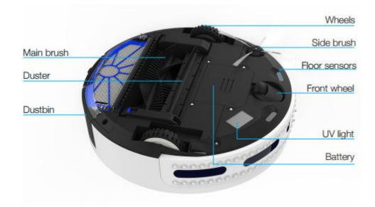
As can be seen in the image above, the side brush has bundles of bristles. On 46. information and belief, these bundles of bristles are positioned such that the bundles pass between the cliff detector and floor surface during rotation, and the bundles are separated by a gap configured to prevent occlusion of the cliff detector beam.
