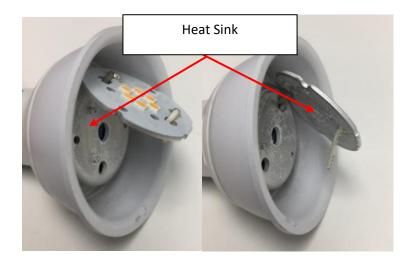
(front and reverse photographs of Euri PAR16 LED Floodlight Bulb with outer cover and inner reflector removed, showing LEDs disposed in heat sink).
