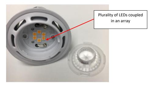
(photograph of Euri PAR16 LED Floodlight Bulb with outer cover removed).
