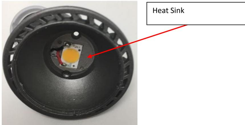
(photograph of Civilight LED HALED MR16 7W Bulb with outer lens and inner reflector removed, showing LEDs disposed in heat sink).
