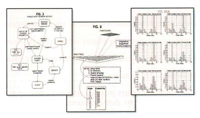
'983 Patent, figs. 3, 8 and 21A (Figures from the patent showing a "schematic representation of a search server residing on a single host computer," a "schematic representation of the C++ Partition object," and a "scores cluster.").
