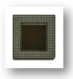
10. A ball grid array is a type of surface-mount packaging (a chip carrier) used for integrated circuits. BGA packages are used to permanently mount devices such as microprocessors. A BGA can provide more interconnection pins than a dual in-line or flat package.
