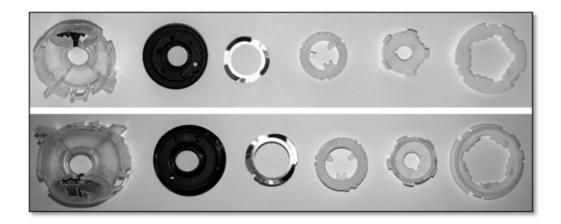
52. The Merck Infringing Products include a first member that is displaceable axially relative to said stationary body. For example, as shown in the images below, the Merck Infringing Products include a castellated white plastic piece that moves axially relative to either the white lid or the lid and the housing.
