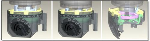
29. The 3M Infringing Products include a stationary body, first member, and second member that are arranged to have a common central longitudinal axis, and the first member is
