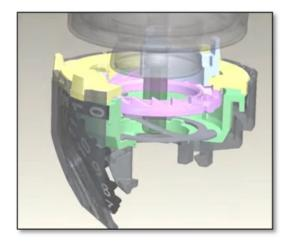
101. The Merck Infringing Products include a counter element in which said counter element includes a second gear co-operating with an actuator gear of an actuator member of the dispenser. For example, as shown in the image below, the saw-toothed ring includes an inner ring of teeth that cooperate with a gear included on the castellated piece.
