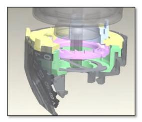
56. The Merck Infringing Products practice each limitation of claim 2 of the '631 Patent. The Merck Infringing Products include a fluid dispenser wherein the second member comprises at least one multi-toothed gear. For example, as shown in the images below, the Merck Infringing Products include a saw-toothed ring with at least one gear containing multiple teeth.
