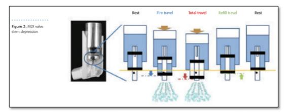
105. The Merck Infringing Products practice each limitation of claim 21 of the '177 Patent. The Merck Infringing Products include a dispenser member wherein the dispenser member is a pump or a valve. For example, as shown in the image below, the Merck Infringing Products include a valve attached to the drug canister for purposes of dispensing the medication.
