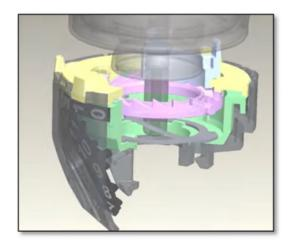
102. The Merck Infringing Products include a second gear in which the teeth of said second gear and/or of said actuator gear are made so that axial displacement of the actuator member causes said counter element to be displaced axially and in rotation. For example, as shown in the images below, the inner ring of teeth on the saw-toothed ring cooperate with the castellated piece, and when the castellated piece moves axially downward, the ring also moves axially downward and rotates.<sup>26</sup>
