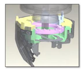
79. The 3M Infringing Products include a second gear in which the teeth of said second gear and/or of said actuator gear are made so that axial displacement of the actuator member causes said counter element to be displaced axially and in rotation. For example, as shown in the images below, the inner ring of teeth on the saw-toothed ring cooperate with the castellated piece, and when the castellated piece moves axially downward, the ring also moves axially downward and rotates.<sup>21</sup>
