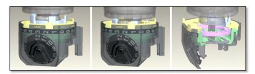
55. The Merck Infringing Products include a stationary body, first member, and second member that are arranged to have a common central longitudinal axis, and the first member is displaceable axially along the central longitudinal axis, and the second member is displaceable axially along <sup>17</sup> the central longitudinal axis and is displaceable rotationally around the central longitudinal axis. For example, as shown in the image below, the lid, castellated
