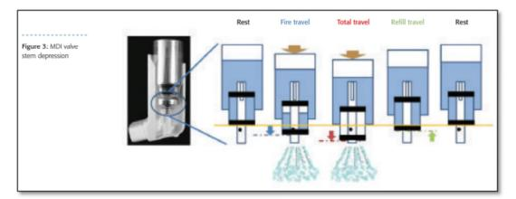
82. The 3M Infringing Products practice each limitation of claim 21 of the '177 Patent. The 3M Infringing Products include a dispenser member wherein the dispenser member is a pump or a valve. For example, as shown in the image below, the 3M Infringing Products include a valve attached to the drug canister for purposes of dispensing the medication.
