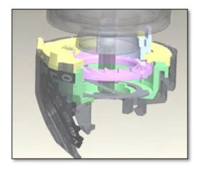
78. The 3M Infringing Products include a counter element in which said counter element includes a second gear co-operating with an actuator gear of an actuator member of the dispenser. For example, as shown in the image below the saw-toothed ring includes an inner ring of teeth that cooperate with a gear included on the castellated piece.
