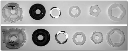
26. The 3M Infringing Products include a first member that is displaceable axially relative to said stationary body. For example, as shown in the images below, the 3M Infringing Products include a castellated white plastic piece that moves axially relative to either the white lid or the lid and the housing.
