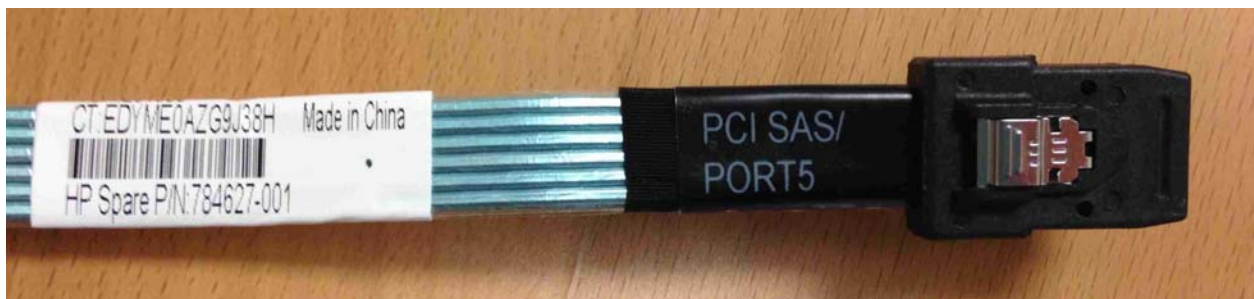
Figure 33. Bottom Side of an exemplary Shielded Ribbon Cable
