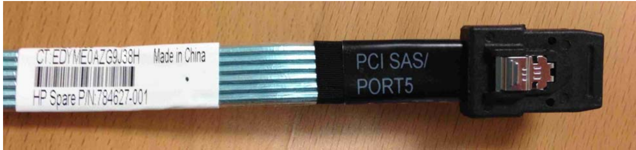
Figure 18. Bottom Side of an exemplary Shielded Ribbon Cable
