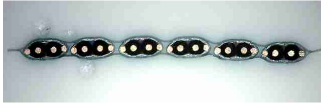
Figure 20. Cross-Section Depicting a Plurality of Conductor Sets
