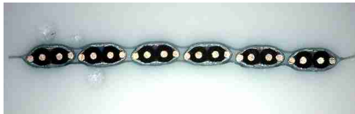
Figure 35. Cross-Section Depicting a Plurality of Conductor Sets
