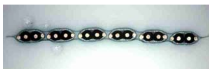
Figure 4. Cross-Section Depicting a Plurality of Differential Pairs
