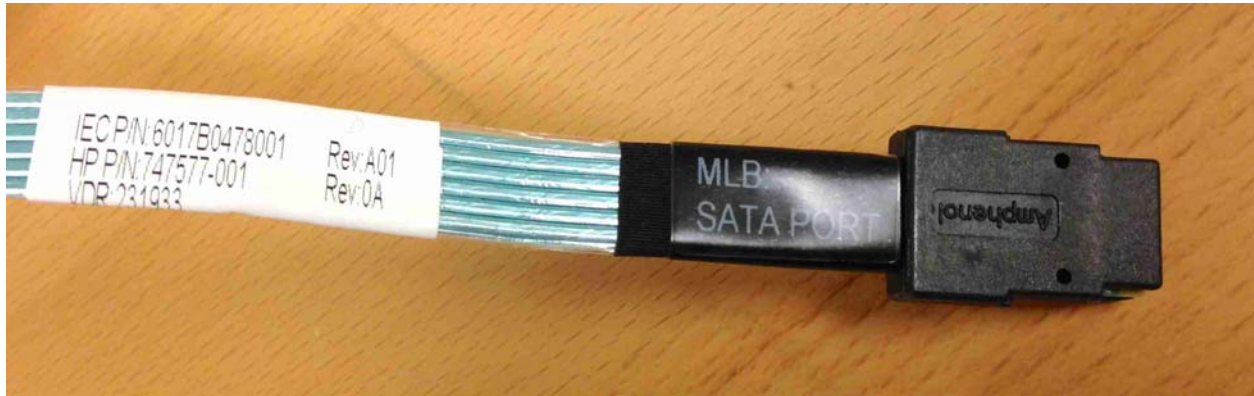
Figure 32. Top Side of an exemplary Shielded Ribbon Cable
