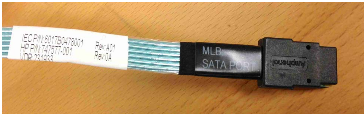
Figure 17. Top Side of an exemplary Shielded Ribbon Cable
