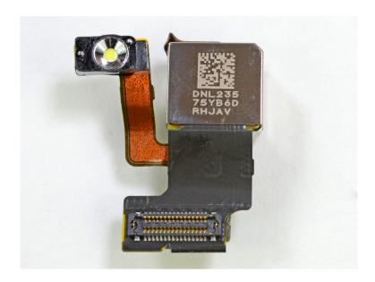
9. The iPhone 5S also utilizes at least one image sensor supplied by either one or more of the Sony Defendants. For example, a teardown of an Apple iPhone 5S also reveals that Sony supplies a camera (8.0 megapixels) having a CMOS construction, as the below photograph illustrates:
