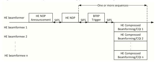
Figure 26-7—An example of the sounding protocol with more than one HE beamformee
